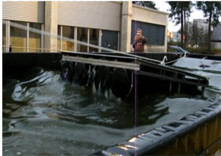
Fig. 23: Experimental investigations of water wave's imitation and pontoons moving. IfSB, BTU Cottbus-Senftenberg
