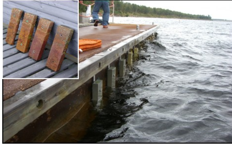
Fig. 22: Concrete samples produced by different concrete formulation after two years contact with water in lake of the former opencast mine
