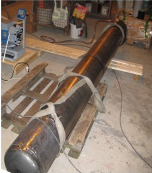
Fig. 18: Heat pipe of vertical beam for predicting of water freezing Fig.: 19: Scheme of heat pipe
